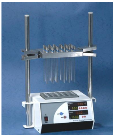
SC-2800D 吹氮濃縮加熱裝置
