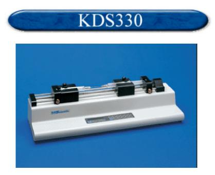
The model KDS330 is designed to emulsify viscous fluids/suspensions by forcing them back and forth through a micro-emulsifying needle. The pump eliminates the fatigue and time required to manually prepare the emulsion.
