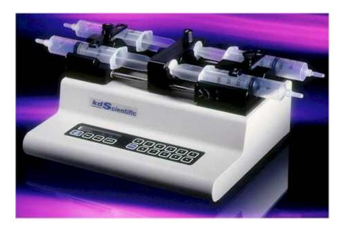
**Push-Pull Syringe Pumps.** This KDS pump provides simultaneous infusio and withdrawal with opposing syringes on a single drive. The KDS260 is an adaption of the KDS210. The pump has been modified to hold an additional syringe so that as one syringe infuses, while the second syringe withdraws at the same rate. **The Push/Pull mode is designed for one cycle only.**
