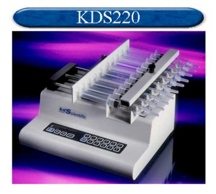
KDS 220 Multi-Syringe Infusion Pump Ideal for applications requiring multiple syringes, the KDS220. Each has been modified to hold up to 10 syringes.
