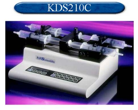
**Continuous Cycle Syringe Pump.** The KDS210C can hold up to four syringes and can cycle continuously back and forth in a push-pull action. As two syringes are infusing, two syringes are withdrawing at the same rate. At the end of the set volume the direction is automatically reversed and the next cycle begins. With the use of 3-way valves the pump can empty and refill syringes for a continuous dispense.
