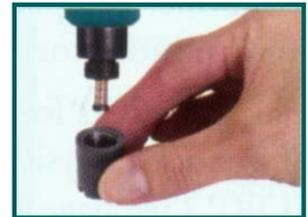
DO sensor with easy to replace screw on membrane cap assembly
